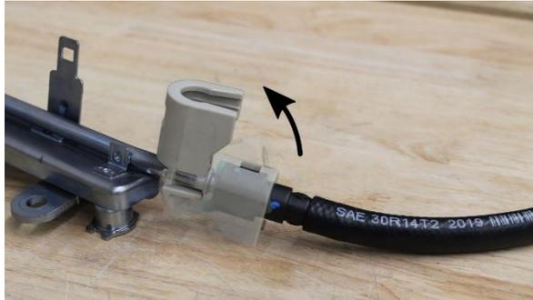
4. Check the fuel quick-connect fittings for dirt (clean if needed) and proceed by placing a rag or shop towel over the quick-connect fitting.
