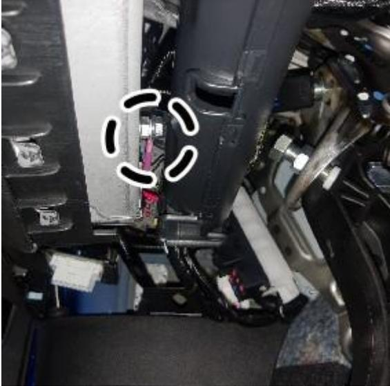
4. Route the 3-Pin Grey Connector from the Chassis Harness to the area you will be installing the Ethanol Gauge. It can be tucked away underneath the dash to draw less attention, or it can be mounted with the supplied gauge pod to a number of locations. One good mounting location is on the center console.
