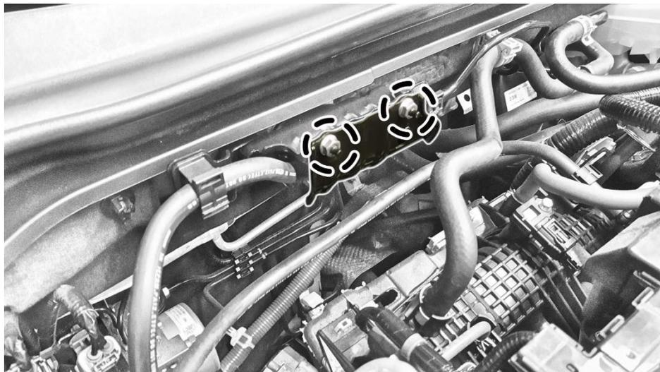
3. Remove the fuel line/quick-connect fitting cover (if equipped).
