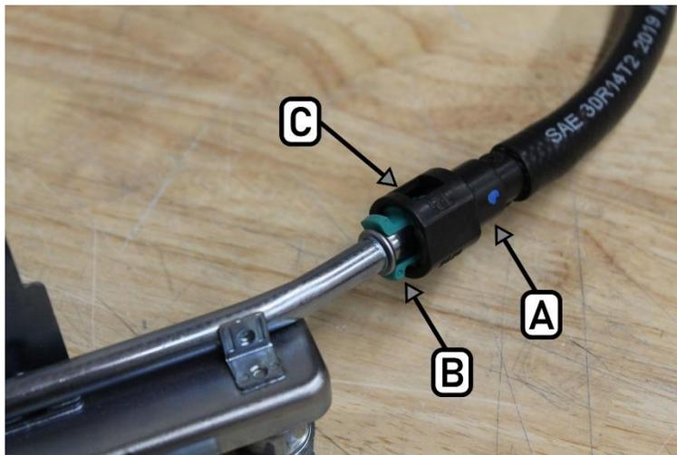
6. Pull the connector (A) and disconnect the fitting.
