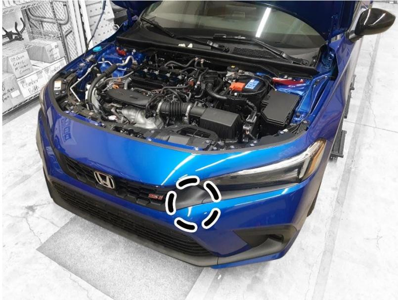
3. Disconnect the vehicle harness connector to the ECT2 Sensor (do not remove the sensor unit from the radiator).
