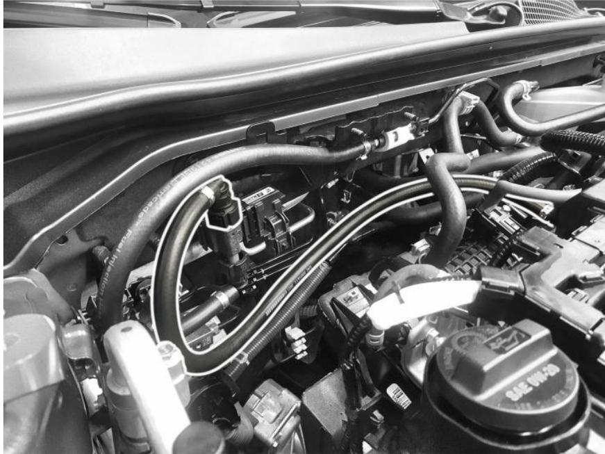
14. Wait to install the fuel hose cover until the entire kit has been installed and the vehicle can run, to check for potential leaks.
