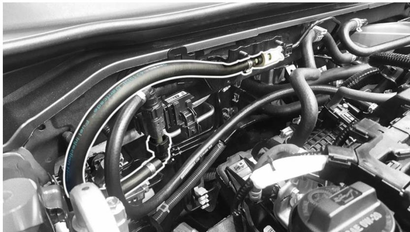
13. Install the longer of the two hoses from the Ethanol Content Sensor to the inlet on the High-Pressure Fuel Pump found on the engine.
