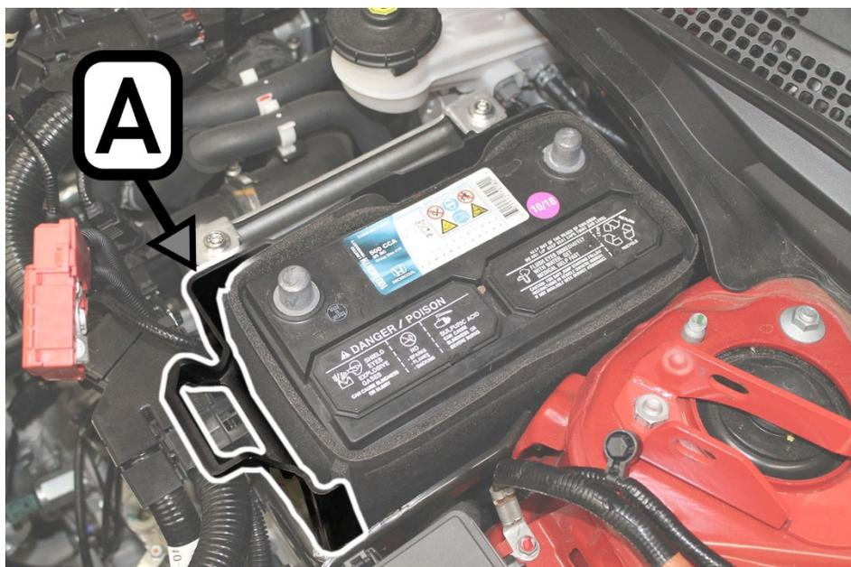
3. Remove Airbox Assembly by removing the 2x 10mm Hex Head Bolts (A), loosening the Inlet Tube Hose Clamp (B) and unclipping the MAF Sensor Harness (C).
